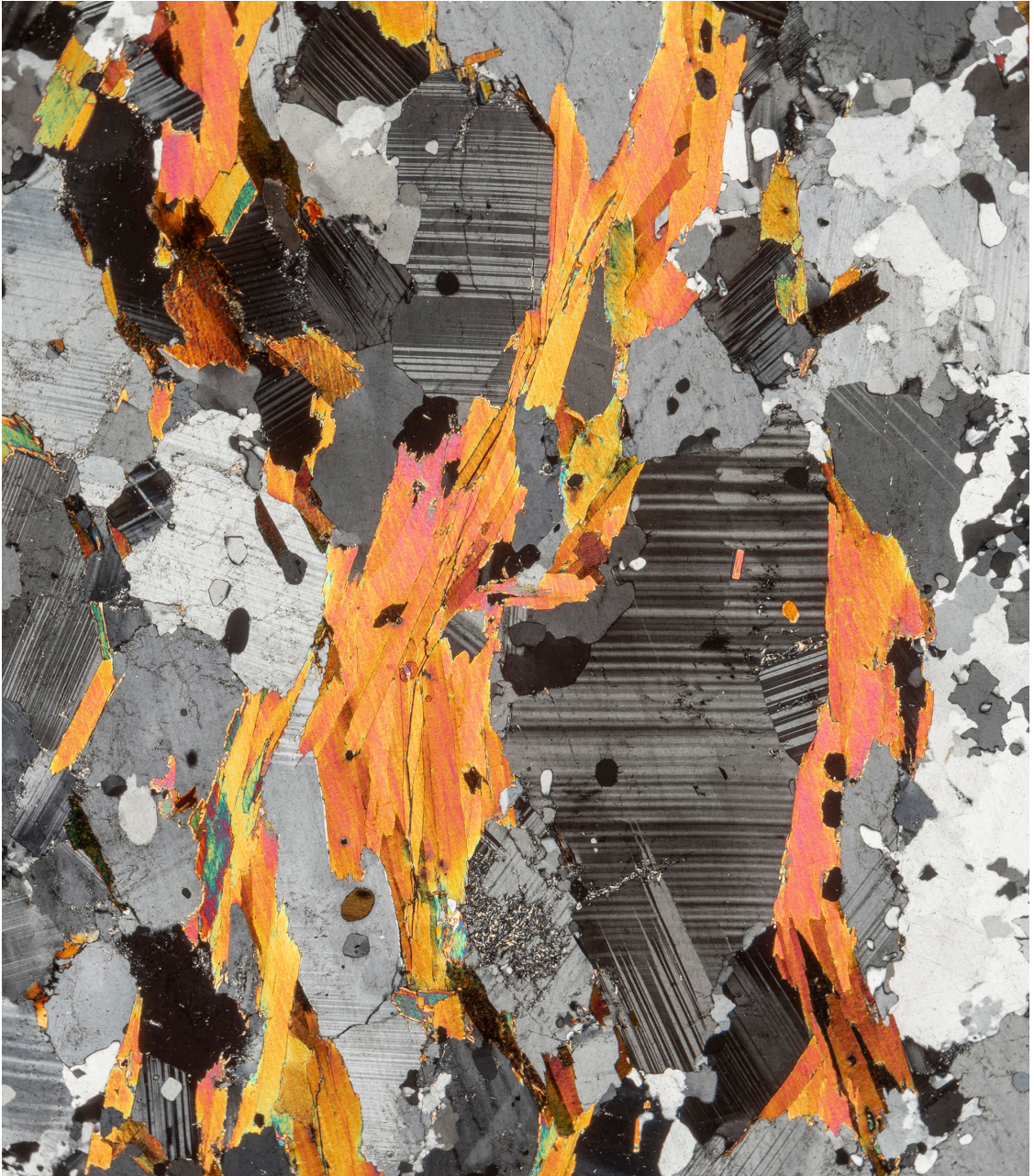
Gneiss. This rock is a common and widely distributed type of metamorphic rock. For microscopic analyses the stone is thin sectioned and polished to 30\mu\text{m} . Polarized light gives information of its mineral content. Light microscope, 27:1
