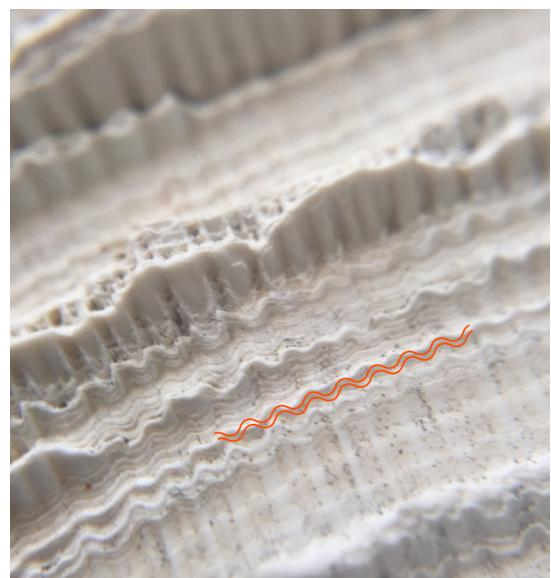
software for 3D printers that allowed us to print ordinary objects using this corrugation method, in one and two dimensions. As expected, the objects were less prone to shearing. However, they were also stiffer overall – something we had not predicted. By simply trying to break the objects by hand (compared to objects made with conventional parallel layers), we sensed that we may have discovered something useful.
