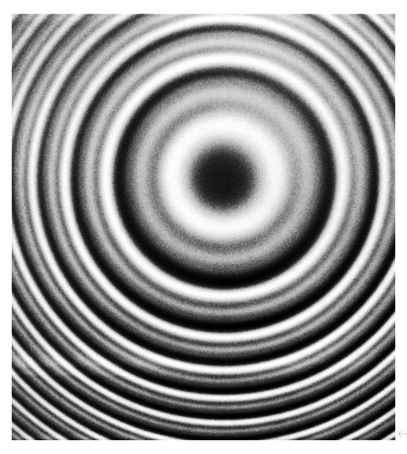
Fabry-perot interferometer/etalon fringes produced using a supercooled, deuterium light source, showing fine structure Photo: Johnwalton, 2007 | Wikimedia Commons
