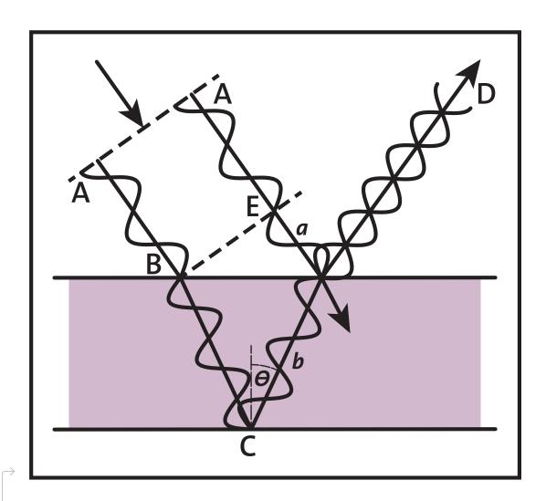
Interference of light waves reflected from front and back
