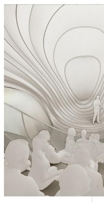
BioRock Pavilion, interior view. Exploration studied the morphology of shells and mathematical surfaces to develop an idea for a pavilion that could accommodate small spoken word performances. The design process started by defining the fixed elements – the seating rake, a stage and a surface for projection – and then used parametric design tools to extend and distort the geometry of the seating into a complete enclosure | Images courtesy of Exploration
