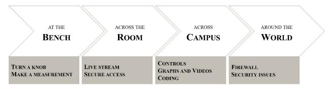
The initial step (at the bench) was to determine whether we could actuate a knob on an apparatus (specifically a power supply) and record data from a sensor. We achieved a positive result at this level by using open-source programmable microprocessors (Arduinos) to control stepper motors and an adapter that allowed the microprocessor to collect the data from the sensor.
