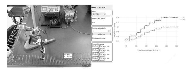
*Note.* Figure 2 shows the screenshot of the lab's web interface. The visual of the experimental set up is shown on the left. The middle section shows the type of the view, users present at the bench, the current settings and the log of actions taken by the users throughout the laboratory period. The right-hand side shows the visual record of the magnetic field values recorded by the sensors.
