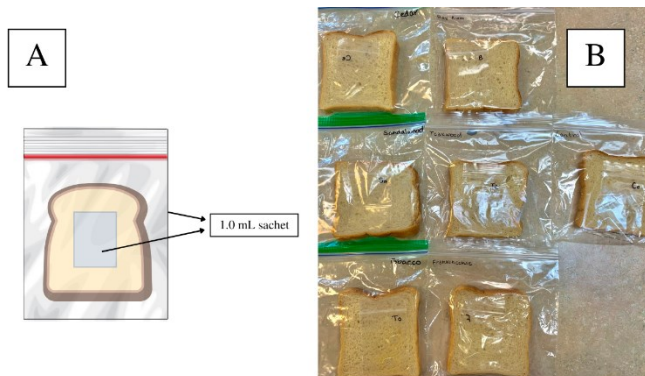
Fig. 1. (A) Depiction of packaging system with an essential oil sachet of 1.0 mL volume placed on either side of each bread slice. (B) Experimental set-up containing six tested essential oils and the control group (center rightmost package).
