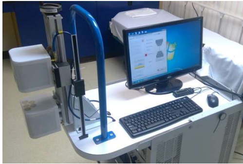
Figure 1: Microwave Transmission system consisting of two sensor arrays and its user interface on a cart. The upper and lower array encloses five ultra-wideband antennas each, distributed in a honeycomb pattern.
