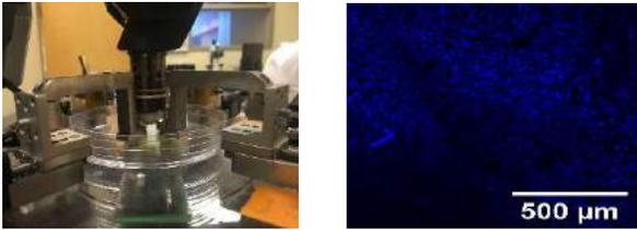
**Figure 1:** Left - coupled mini-biaxial machine and confocal microscope system. Right - confocally imaged porcine aorta sample with stained nuclei midway through modified biaxial test.
