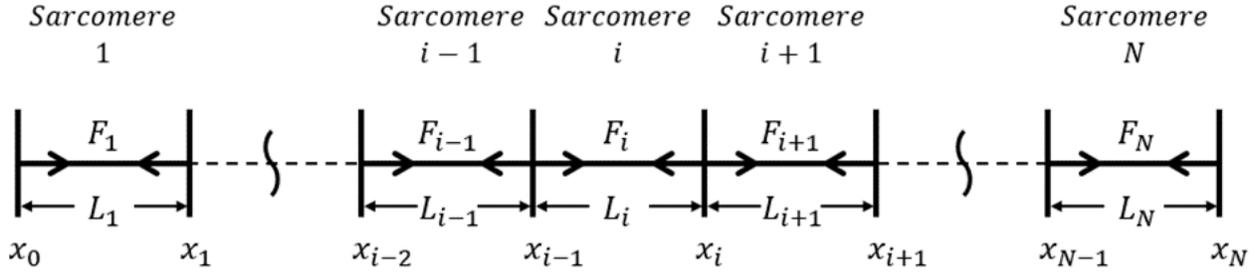
**Figure 4:** Variable definitions for models.  $F$  is the sarcomere force produced from the  $i$ th sarcomere,  $L$  is the length of the  $i$ th sarcomere, and  $x$  is the total distance of the  $i$ th sarcomere from the start of the myofibril.
