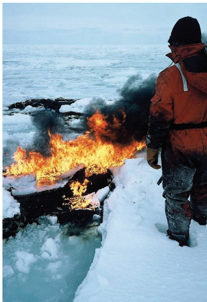
FIG. 10. Burning thick oil contained in a slush-filled lead off Nova Scotia in 1986 (Photo: D. Dickins).
