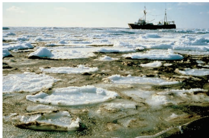
FIG. 8. Oil in slush between pancakes in a dynamic ice environment after the first release off Nova Scotia, 1986. The support vessel Brandal in the background (Photo: Environment Canada).
