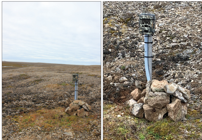
FIG. 2. Example setup of the Reconyx HyperFire outdoor camera (Photos: A. Robinson).
