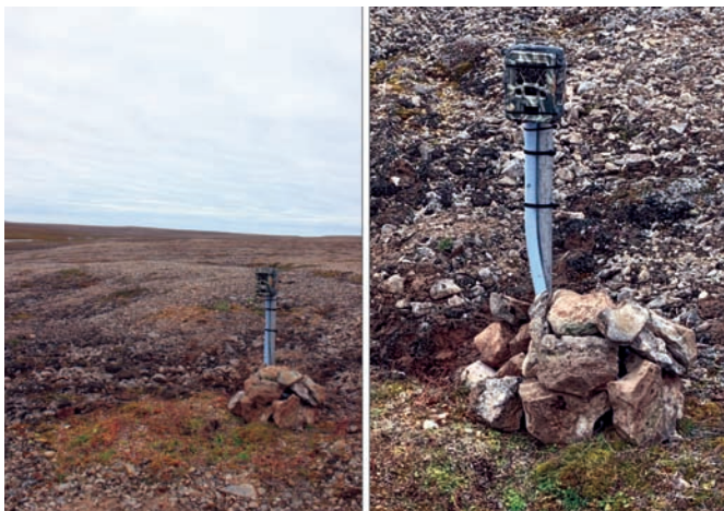
FIG. 2. Example set-up of the Reconyx Hyperfire Outdoor camera. Photo: A. Robinson.
