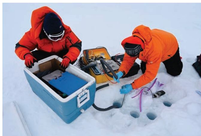
FIG. 2. Taichi Noshiro (Japan, left) and Bruno Delille (Belgium, right) collect sea ice brine chemistry samples to compare different sampling and analysis techniques. Photo: Daiki Nomura.
