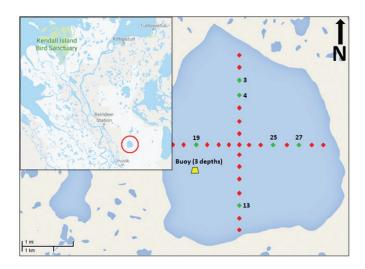
FIG. 4. Schematic representation of locations for the ice survey (red diamonds) and water sampling (green diamonds) in Noell Lake. Additional water samples were taken at a site near the ALMS Buoy (yellow trapezoid). The inset shows the location of Noell Lake (circled in red) in the context of Inuvik, NWT, and the Mackenzie Delta uplands.
