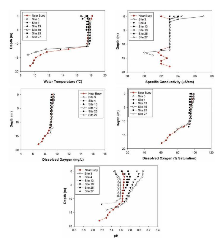
FIG. 8. Open-water depth profiles of a multitude of limnological parameters recorded by a hand-held water quality sonde at a multitude of locations in Noell Lake on 8 August 2012.
