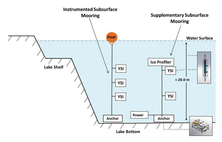
FIG. 3. Schematic representation of the supplementary subsurface mooring (right) and instrumented subsurface mooring (left) deployed in Noell Lake, NWT. Yellow Springs Instruments, water quality sonde.
