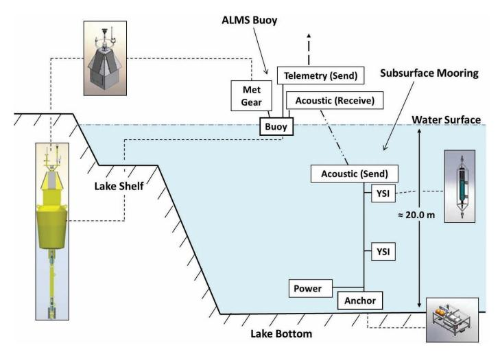
FIG. 2. Schematic representation of the ALMS buoy and subsurface mooring system deployed in Noell Lake, NWT. Meteorological (Met) Gear: Anemometer – windspeed; temperature and relative humidity sensors; pyranometer – radiation; barometer – pressure. Yellow Springs Instruments, water quality sonde.
