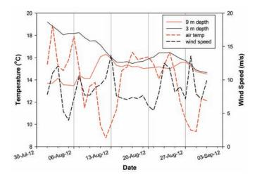
FIG. 11. Time series of air temperature (°C) and wind speed (m/s), as measured by the Inuvik Airport Weather Station, and water temperature (°C) measured at 3 m and 9 m below the water surface.
