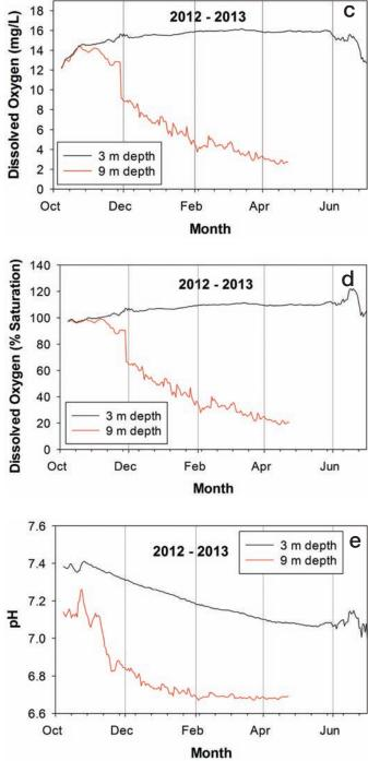
FIG. 6. Plots of continuous limnological measurements recorded by various buoy and mooring components of the Arctic Lake Monitoring System during several under-ice periods. The black line represents parameter values recorded at a depth of 3 m below the water surface. The red line represents parameter values recorded at a depth of 9 m below the water surface.
