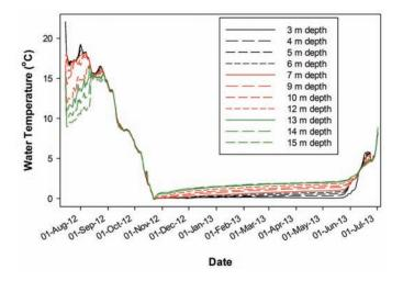
FIG. 7. Time series of water temperatures recorded by HOBO data loggers strapped at 1 m intervals to the cable of the instrumented subsurface mooring.
