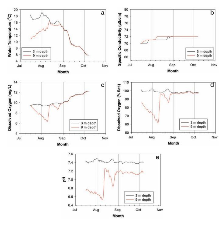
FIG. 5. Plots of continuous limnological measurements recorded by various buoy and mooring components of the Arctic Lake Monitoring System during the 2012 open-water period. The black line represents parameter values recorded at a depth of 3 m below the water surface. The red line represents parameter values recorded at a depth of 9 m below the water surface.
