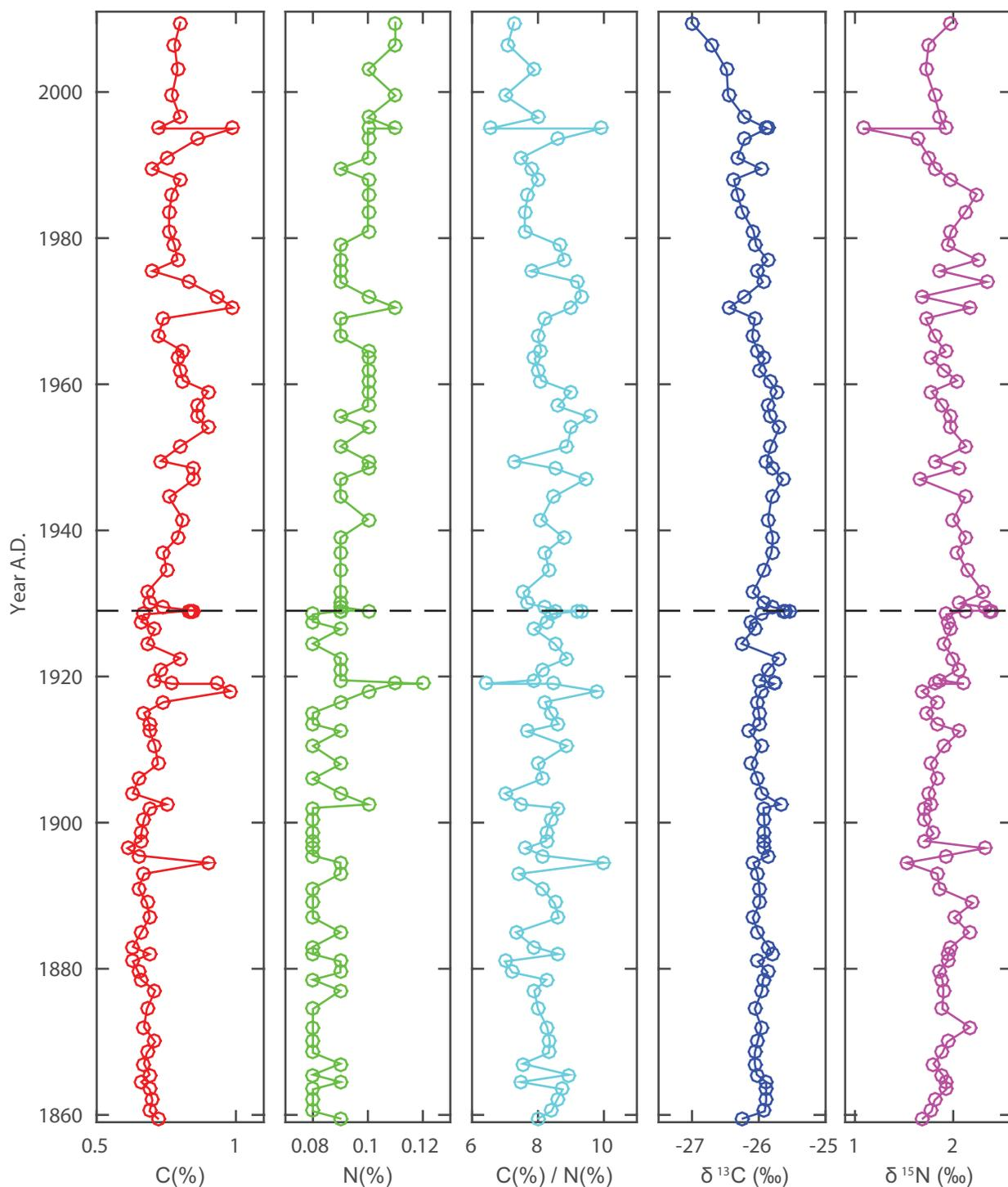
FIG. 5. Geochemical results from core EK 12-01 at Eklutna Lake. Values are plotted against the average year of deposition of each 1 cm<sup>3</sup> sample. The dashed horizontal line emphasizes the date (1929) when the first dam was installed on the Eklutna River.
