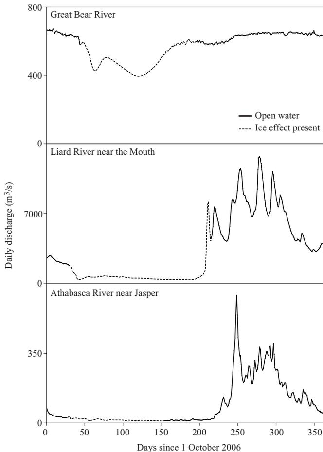
FIG. 4. Hydrographs of the Great Bear River, the Liard River near the mouth at Fort Simpson, and the Athabasca River near Jasper for 2006–07, showing differences in the length of the ice-effect period.
