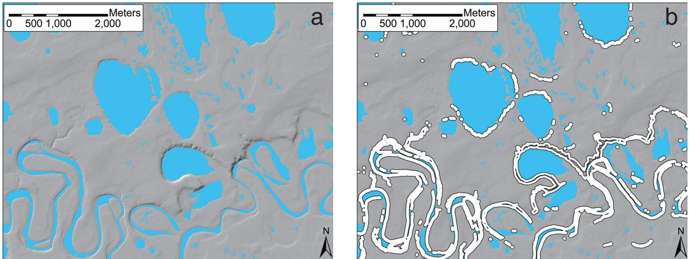
FIG. 4. Examples of IfSAR DTM data in the National Petroleum Reserve – Alaska. (a) Hill shading is used to increase the visibility of terrain changes. Abrupt changes in landscape are indicated by extreme dark or extreme light shading. (b) Polar bear denning habitat, identified by white lines highlighted with a black border, occurred mostly along stream banks and lakeshores.
