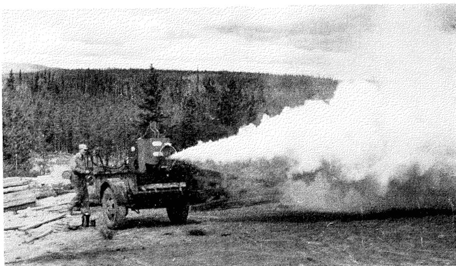
**Plate 10.** Aerosol generator mounted on vehicle discharging insecticide in control experiments against black flies and mosquitoes at Whitehorse.
