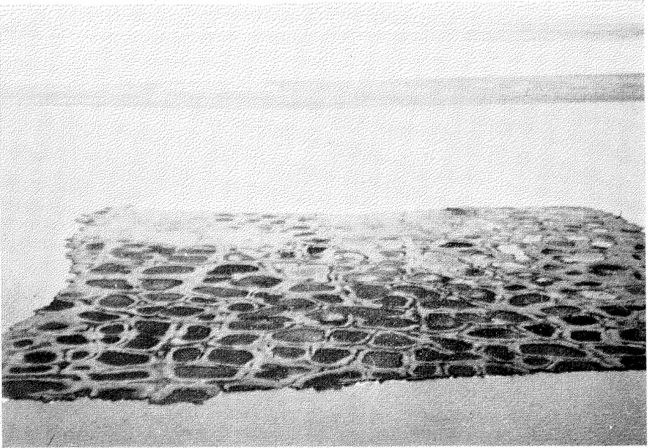
Fig. 4. Island of polygonal ground near Dease Inlet. Note the details of the shoreline following the ice wedges. All polygons shown are of the "low-centred" type. 24 July 1950.
