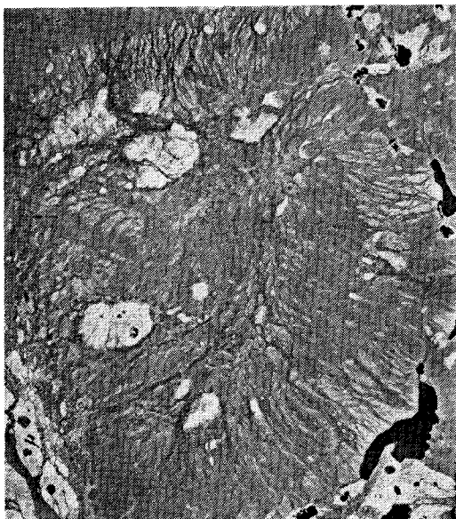
FIG. 5 Domed macrorelief structure showing the variation of type of linear-patterned slope with aspect, the pattern associated with near-surface permafrost occurring mostly on NNW- to SE-facing slopes, and the pattern not associated with near-surface permafrost occurring mostly on SSE- to W-facing slopes (part of air photograph A12599-248, Air Photo Division, Dept. of Energy, Mines and Resources, Canadian Government copyright, scale 1:63360, with north towards top of page).
