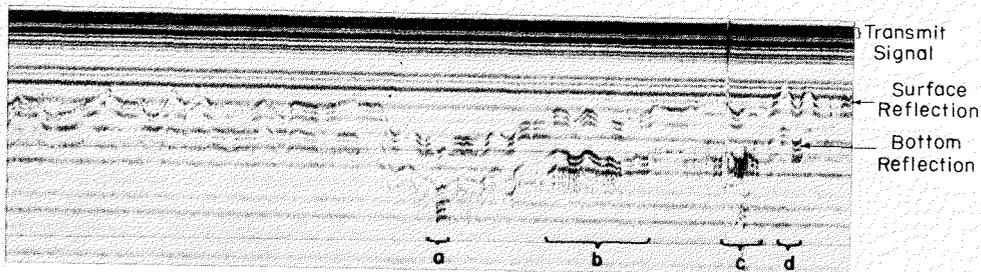
FIG. 10. Impulse radar record obtained along the helicopter sounding flight path shown in Figure 9 on Big Lake. The "bright spots," dark areas on the record, indicate potential sites where water still exists under the ice.
