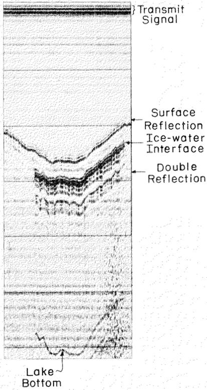
FIG. 8. Impulse radar record obtained during a helicopter sounding flight down the long axis of Webster Lake.
