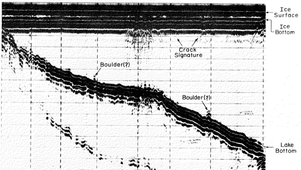
FIG. 2. Radar sounding data taken from the ice surface on Canaan Street Lake, Canaan, New Hampshire. The record shows interfaces and other detail typically obtained during impulse radar profiling on freshwater ice. The distance between vertical event marks is 20 m.
