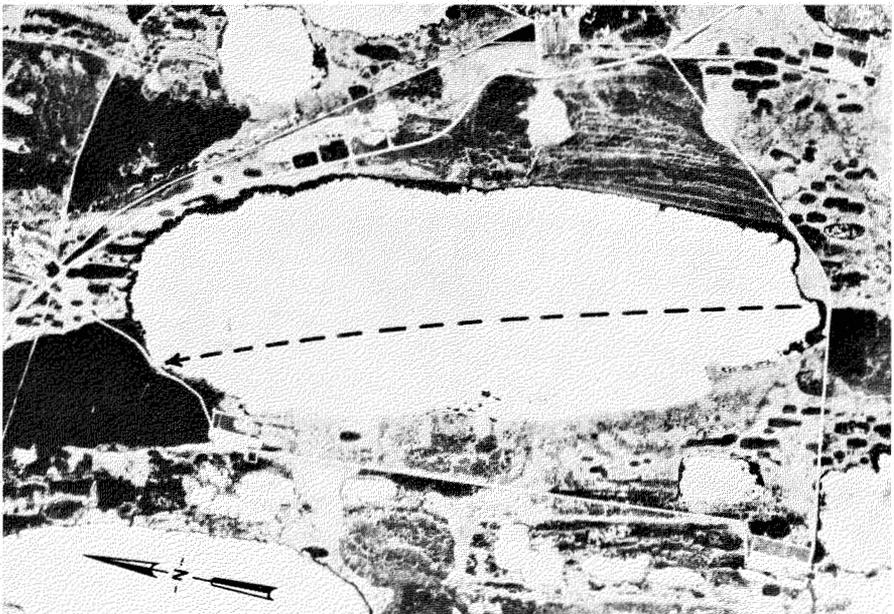
FIG. 9. Big Lake and the flight path taken during impulse radar sounding. The British Petroleum camp complex can be seen across the road on the east side of the lake.
