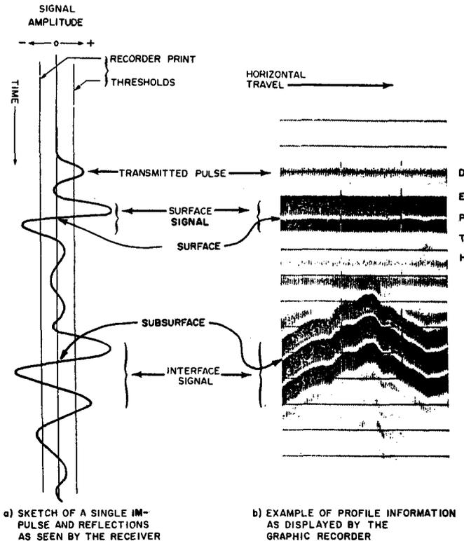
FIG. 1. An example of the radar impulse signal versus time and its equivalent real time graphic recorder display.
