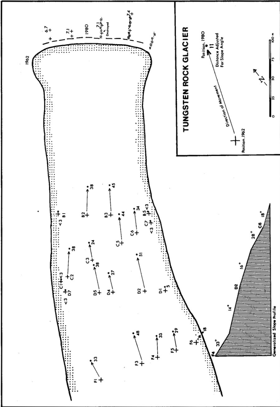
FIG. 3. Map showing the initial and present positions of marked boulders. The crosses below the snout indicate the positions of previously surveyed trees. The adjacent numbers indicate the distance of movement of the snout immediately adjacent to the trees. An active spring presently discharges from the rock glacier and the resulting stream flows past the tree marked by 7.4 m. Two presently inactive springs and stream beds are present on either side.
