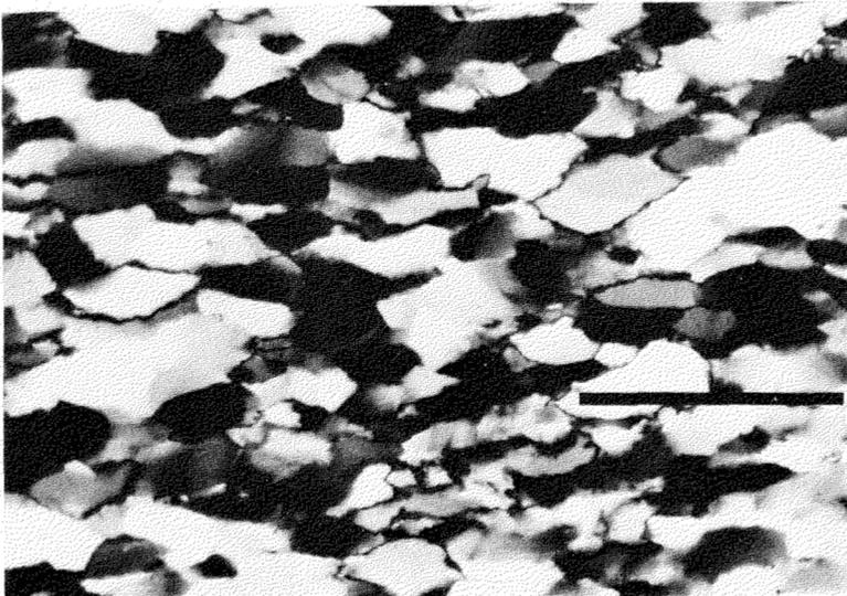
FIG. 6. Photomicrograph, Ramah Chert — sample #77-4. Note the deformation of the quartz grains. Bar scale 0.1 mm. Photo: C. Lazenby
