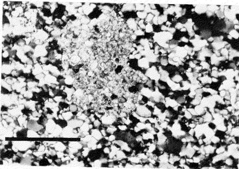
FIG. 7. Photomicrograph, Cod Island chert-sample #77-8. Note the small size of the grains and the absence of deformation. Large grain in the centre is a carbonate. Bar scale = 0.1 mm. Photo: C. Lazenby.
