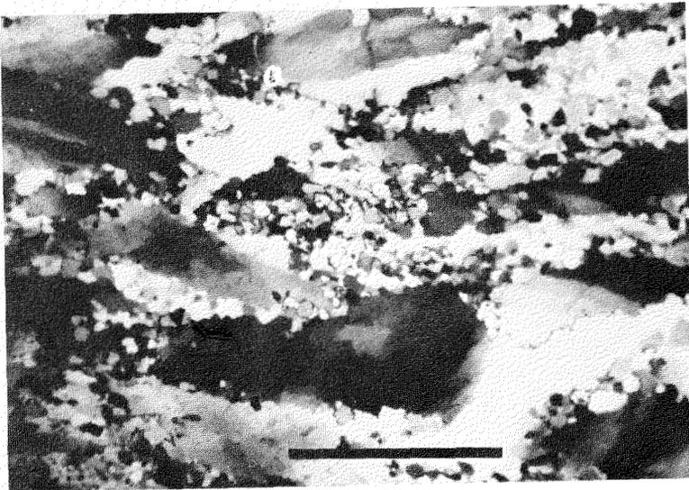
FIG. 8. Photomicrograph, Ryan's Quartz — sample #RB-1. Note fine grains dispersed among larger ones. Bar scale = 0.29 mm. Photo: C. Lazenby
