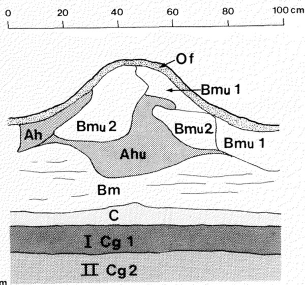
FIG. 3. Soil profile of an earth hummock at T-25 in the Sunshine area. The subscript 'u' indicates turbation.
