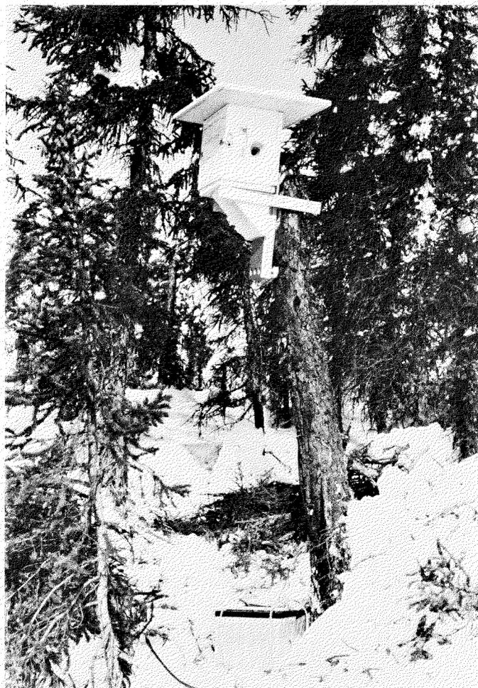
FIG. 13. Time-lapse camera system installed on a tree; main batteries visible at the base of the tree.
