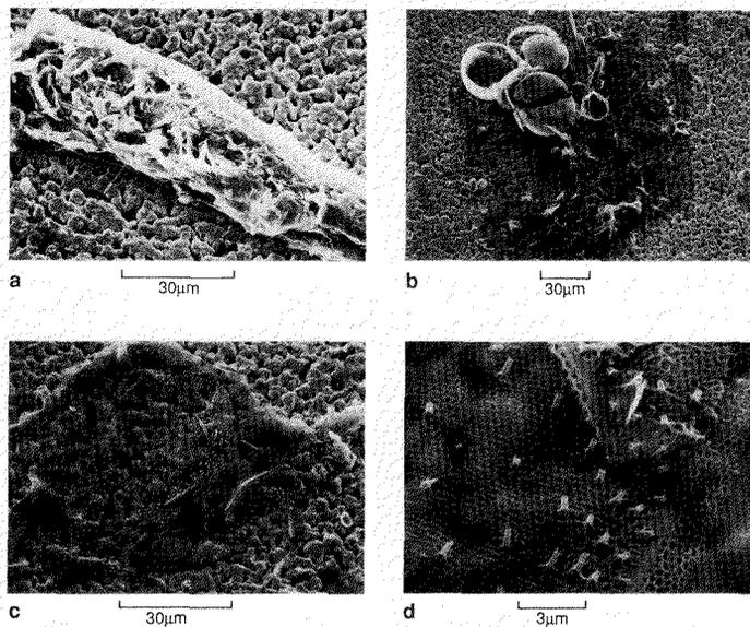
FIG. 7. Scanning electron micrographs of SPM particles: a) Si-rich (98%) fecal pellet from 30 m of water at Station 6; b) large mucoid agglomerate with remnant diatoms from 30 m of water at Station 6; c) mucoid (possibly from a flagellate) with the internal structure preserved, from 10 m of water at Station 8; d) close-up of "c". The background, which is apparent in the SEM pictures, is the matrix of the silver filters.
