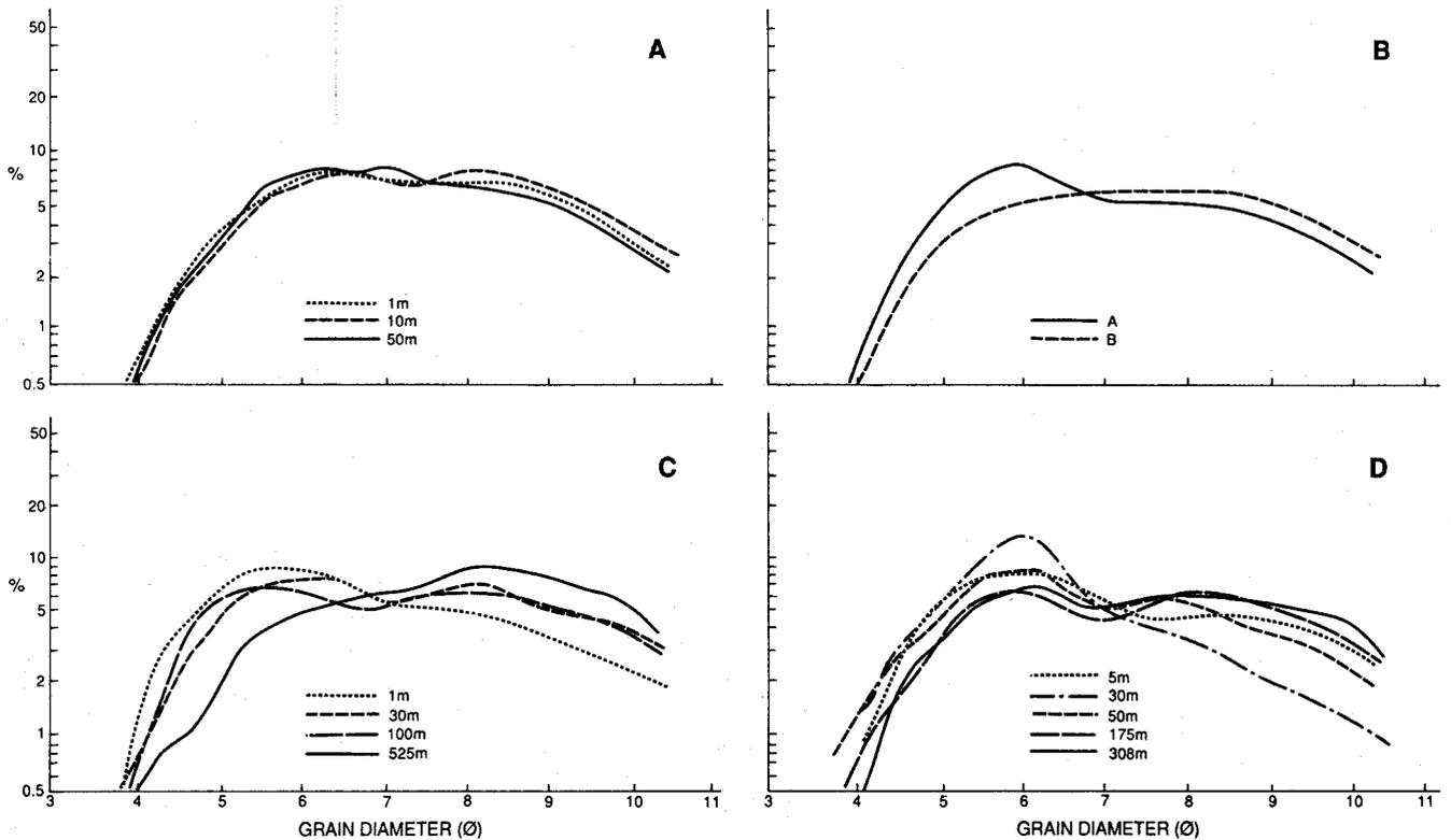
FIG. 10. Suspended sediment size frequency distributions for 29 and 30 September and 1 October 1983 from: A) Station 0.1c at depths 1, 10 and 50 m; B) average surface water observations, A, and average bottom water observations, B, for all stations; C) Station 3.05 at depths 1, 30, 100 and 525 m; and D) Station 2.1B at depths 5, 30, 50, 175 and 308 m.
