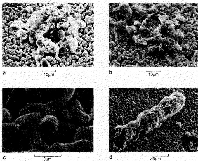
FIG. 6. Scanning electron micrographs of SPM particles: a) floccule of diatoms and phyllosilicates from 50 m of water at Station 1; b) inorganic floccule with a light organic coating from 312 m of water at Station 1; c) picoplankton, 2  $\mu\text{m}$  in diameter, from 20 m of water at Station 3; d) Si-rich fecal pellet from 20 m of water at Station 3. The background, which is apparent on these SEM pictures, is the matrix of the silver filters.
