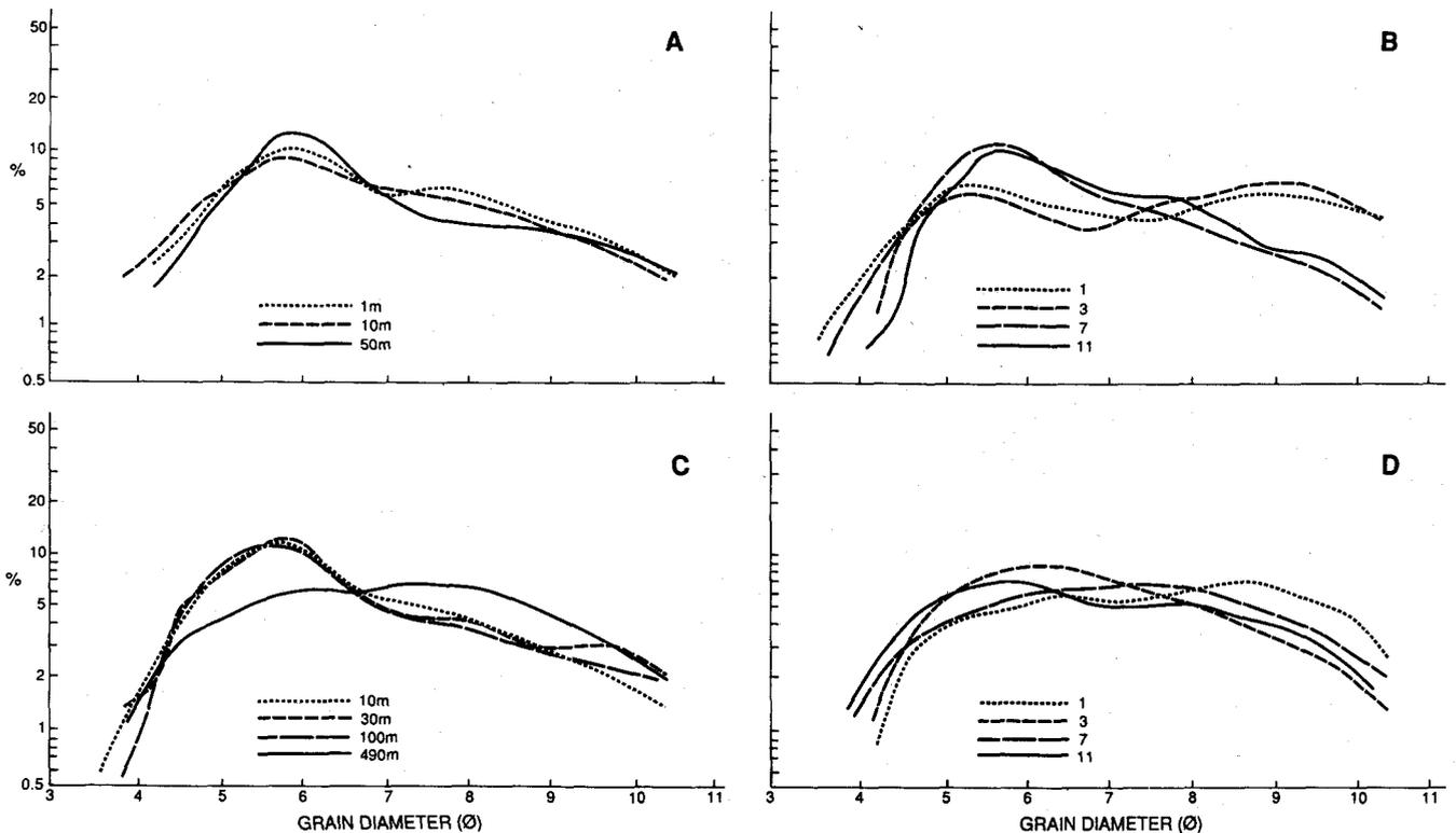
FIG. 9. Suspended sediment size frequency distributions for 18 and 19 September 1982 from: A) Station 6 at depths 1, 10 and 50 m; B) Stations 1, 3, 7 and 11 at a depth of 10 m; C) Station 7 at depths of 10, 30, 100 and 490 m; and D) near-bottom samples for Stations 1 (312 m), 3 (435 m), 7 (490 m) and 11 (241 m).
