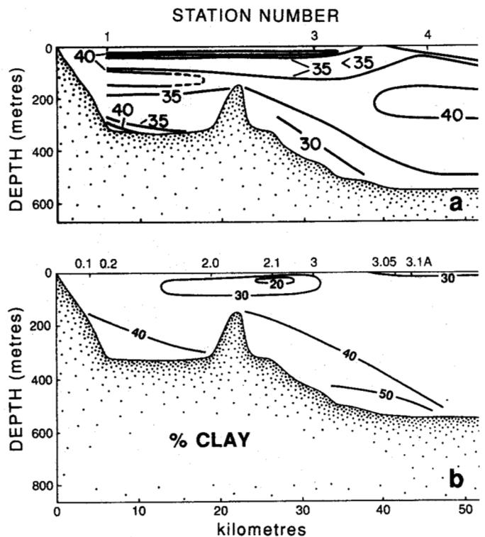
FIG. 12. Percentage of clay determined from textural analyses of the SPM from the inner 50 km of the fiord for the observations made during a) 1982 and b) 1983.
