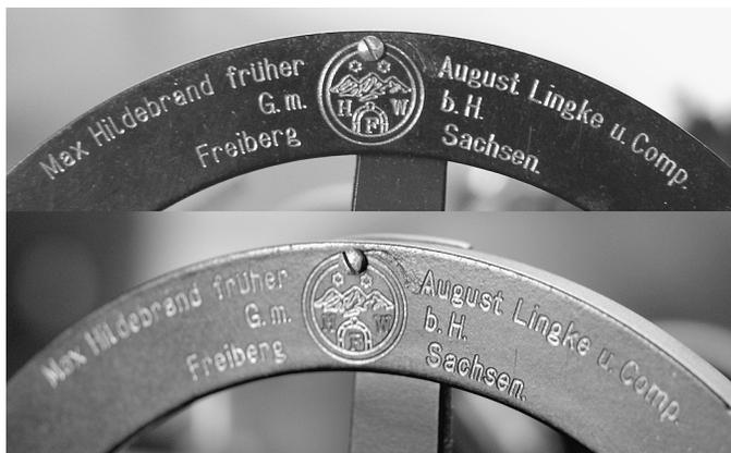
*Details of the Hildebrand trademark on the transit seen from straight on (top) and at a 30° angle. Note the marked difference in appearance of the “H W F” within the circle.*
